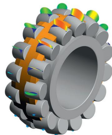
Spherical roller bearing showing progression of contact pressure and slippage
