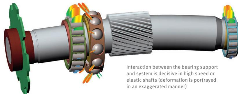
Interaction between the bearing support and system is decisive in high speed or elastic shafts (deformation is portrayed in an exaggerated manner)
