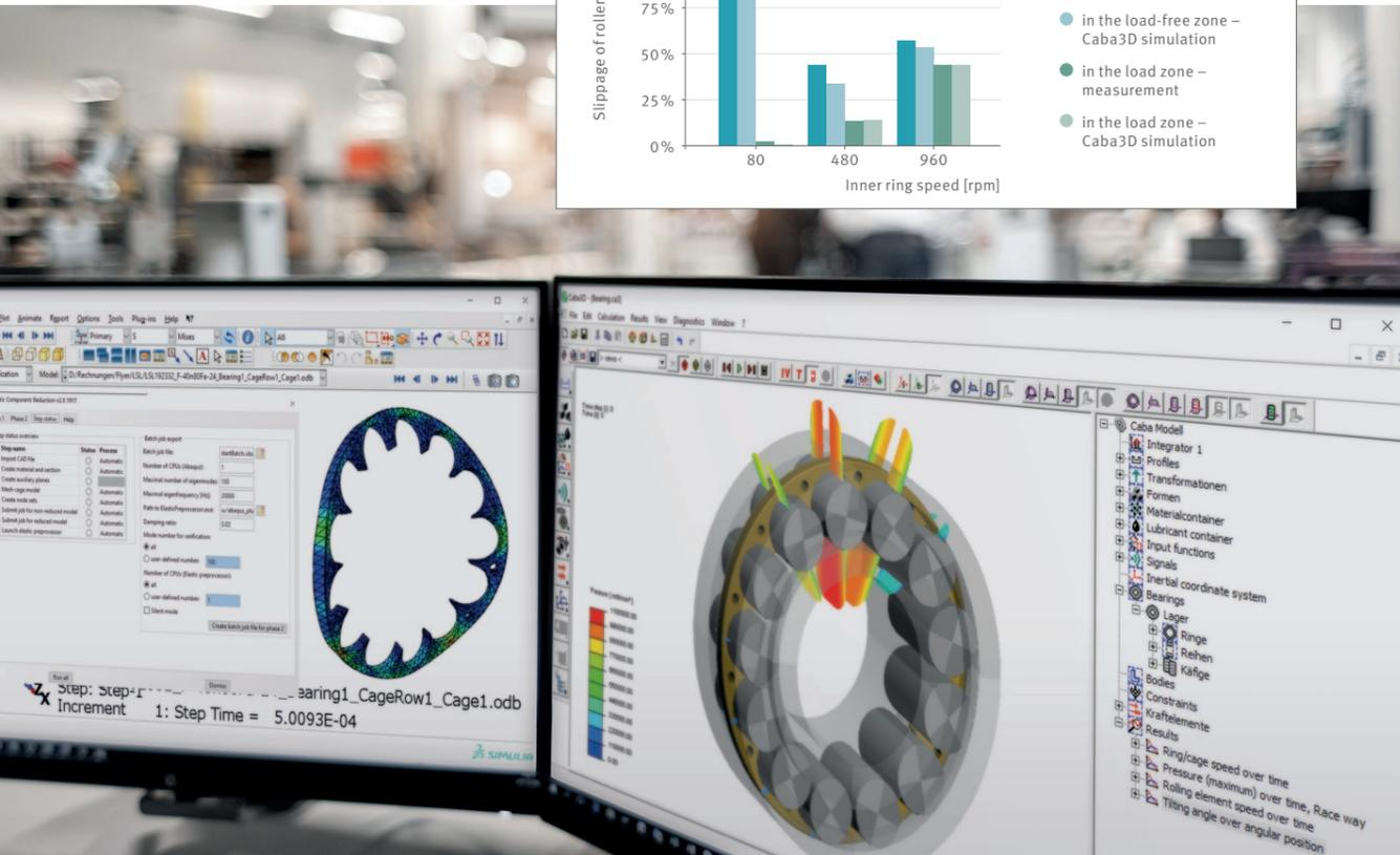
Caba3D is validated using tests and FEM calculations
